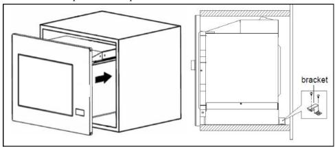
5. Open the door, fix the oven to the cabinet with Screw B, at the installation hole. Then fix the Trimkit plastic cover to the installation hole.
